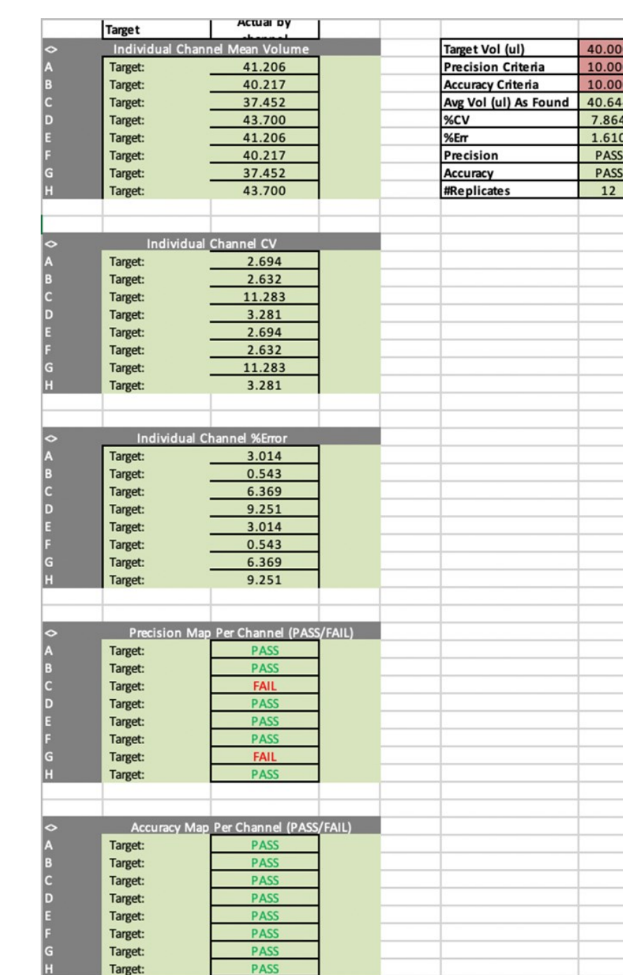
Fig. 7. Volume verification within GLH Tracker software.
